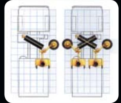
Curbside vacuum nozzle, gutter broom and fixed transfer broom
